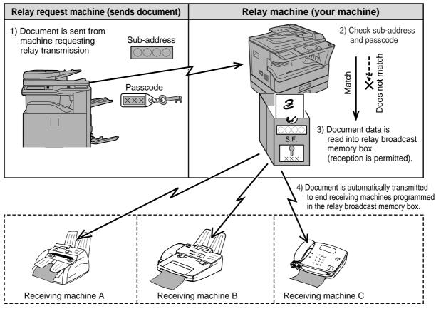
The machine that originally sends the document is called the relay request machine, and the machine that has a memory box containing the end receiving machines and which relays the received document to those machines is called the relay machine.
